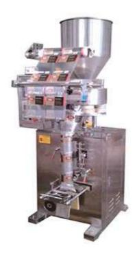
This baler is bag making type, applicable for packing granular products. such as: granulated sugar, salt, potato chips, popcorn, nuts, etc.
