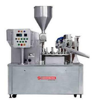
Automatic Tube Filling Machine - Automatic Single head tube filling & labeling machine is precision built on sturdy welded SS frame completely enclosed in stainless steel sheet and doors are providing to facilitate the servicing of machine.
