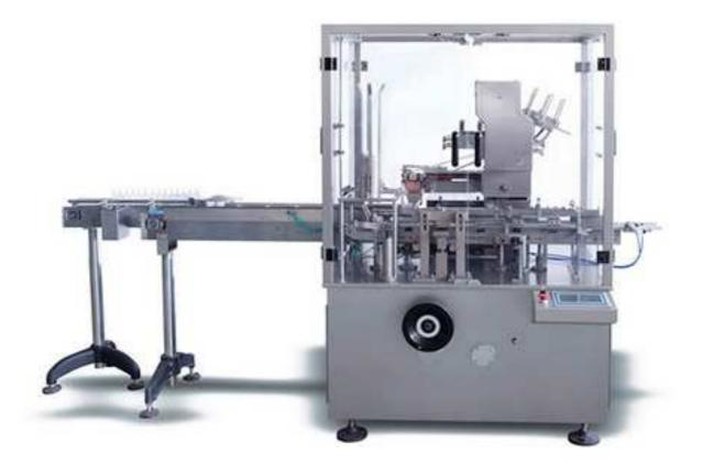
This machine Is suitable for automatic feeding bottle (round, square bottie) into carton (either for blister or bottle). Online bottle unscramble and feeding, leaflet told (1-0tolds) and feeding, leaflet detecting, canton opening and forming, products and leaflet pushing into carton, printing batch number, sealing carton with tuck-in or hot melt glue device. Automatically reject lacking of leaflet or product and finished product out.
