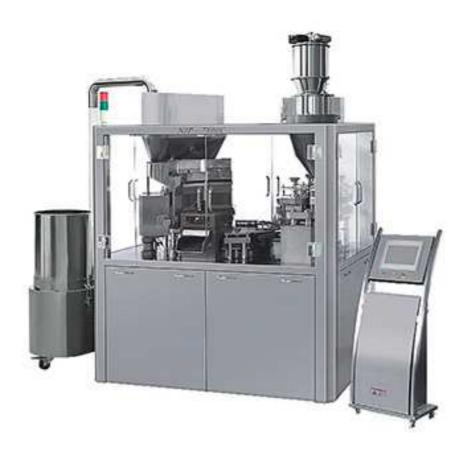
The NJP-7800C provides a high versatility of filling options with varying product types. Even complex products with varying filling parameters can easily be processed, in addition to (micro) tablets, powders, pellets, and granules. With an output of 7800 capsules per minute, this high-speed machine is reliable, low-maintenance, and provides production security.
