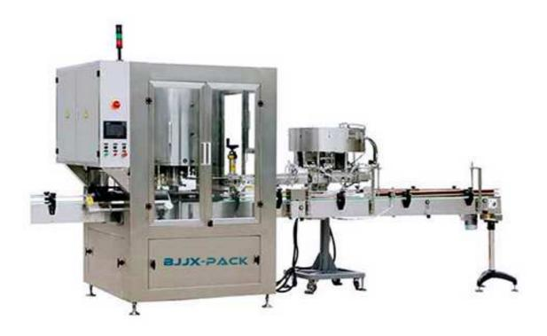
This machine is conveying the bottle to the screw conveyor, and then goes to the star plate to the capping machine, the bottle-chuckle chuck the bottle neck (or the belt strap-ping the bottle) to capping process. Finally through the star plate, the capped bottle conveyed to the next belt. The whole capping process finished.
