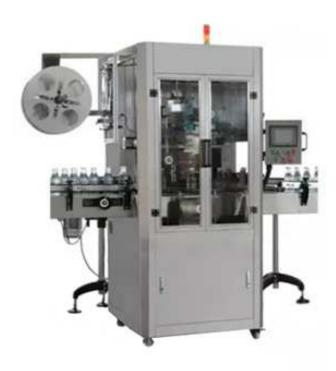
It adopts PLC programmable controller, imported servo motor, servo driver, frequency converter and transducer; Also, it adopts the positioning module to ensure the casting label precise, rapid and stable.
