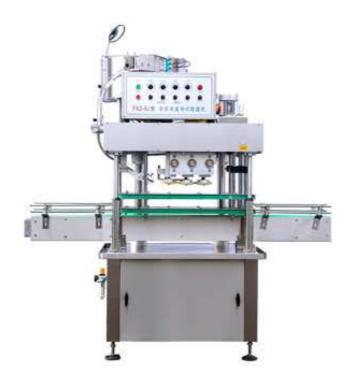
FXZ-6J Automatic linear capping machine includes the bottle tightening conveying structure and capping wheels. Under the horizontal movement of the conveyor, it will finish the complete process of capping. It can be widely used for capping of round and flat bottles. The machine is with simple structure, easy adjustment and quick change-over between different bottles.
