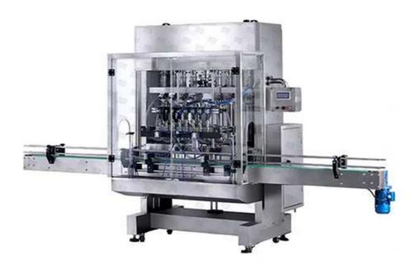
The high-precision 6 head liquid filling machine is a high-tech product developed by our company. It is suitable for water injection, fluid and detergent products with different viscosities. It is widely used in the filling products of food, cosmetics, medicine, oil, daily chemical, detergent, pesticide, chemical industry and other industries. Different types of solutions can be filled without adding any additional parts.
