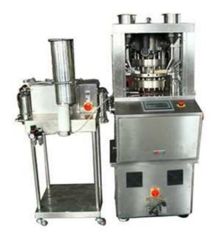
It's apply to used for effervescent, disinfection, sugar tablets and to avoid materials are sticking on moulds, it sprays magnesium stearate to prevent materials from sticking and as lubricating agent to machine.
