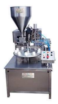
Semi Automatic Single head tube filling Machine is precision built on sturdy welded MS frame completely enclosed in stainless steel sheet and doors are providing to facilitate the servicing of machine.
