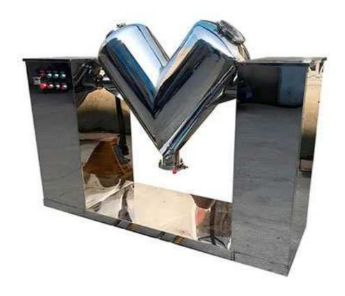
The VI series forced Mixer Machine is equipped with a stirring shaft, which can mix finer powder particles, agglomerated powders or more than two kinds of powders, and materials containing a certain amount of moisture. The Mixing Machine is made of stainless steel 304, and the inner and outer walls of the mixing barrel are polished. This Industrial Blender machine has beautiful appearance and strong practicability, and is widely used in food, pharmaceutical, chemical and other industries.
