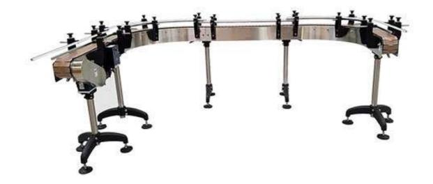
SureKap conveyors are constructed with heavy-duty stainless steel. They are available in most lengths and widths of either 4.5", 7.5" or 10". Each conveyor features a variable speed drive, acetal low friction belt, and adjustable height.
