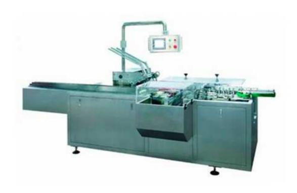
Boxing Packing Machine is automatic high speed continuous cartoning machine which is high performance product incorporates pneumatic, photo, electric, mechanic in one. It suitable for automatic inserting ALU-PVC blister, bottle, soft tube, soft AL/AL strips and pouch into carton, also can link to matching machine to form production line.
