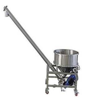
SLJ series spiral round pipe vibration feeder is a kind of economical and practical convenient feeding machine, its characteristic is simple installation, easy to use, maintenance is convenient. Due to the uniqueness of the design, easy to transport liquid and powder material with poor liquidity, such as milk powder, monosodium glutamate, solid drink, white sugar, dextrose, coffee, feed, pharmaceutical, pesticide, solid powder, granular additive, dyestuff, etc.
