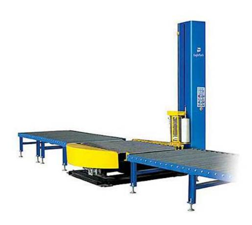
This machine have powered out feed conveyor and powered conveyor zed turntable system and is able to transport an wrapped load from the turntable to the out feed conveyor if there is no wrapped load on the out feed conveyor. The film cutting and clamping unit and the tail wipe system provide a fully automatic wrapping cycle and adherence of the film to the load.
