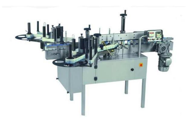
Automatic Double Side Sticker Labeling Machine Is Used To Apply Label On Model NKSAL - 120D Is Suitable For Applying Front And Back Labels On Flat/Oval/Square/Round Shape Containers With Output Up to 120 Labels Per Minute Depending On Products And Label Size.
