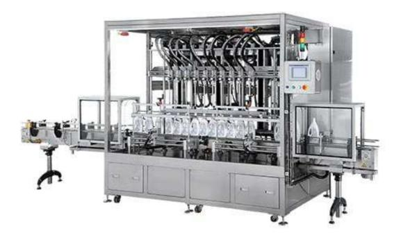
FL serials are volumetric filler, it works with various types and shapes of packages and a wide range of liquid material, this future designs and advancing technology filling system is cable of filling thin and foamy liquid.
