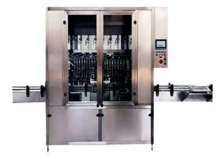
The machine adopts servo-piston filling mode which are mainly used for various of viscosity agent and good fluidity material. Applicable to food, daily chemical, cosmetic, oil and the other industries with relatively high demand for production capacity requirements.
