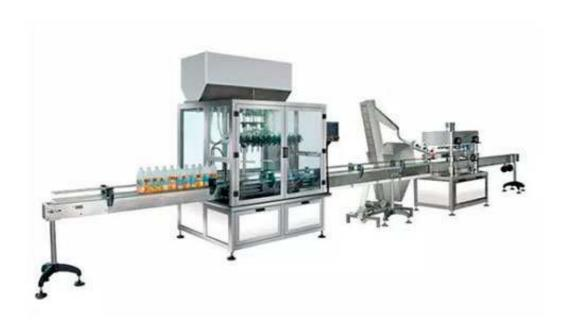
Automatic Shampoo Filling Machine is suitable for filling soybean oil, peanut oil, tea oil, beverage, mineral water, juice beverage, lubricating oil, oil, laundry liquid, detergent and other liquids and oils, and is not limited by bottle type.
