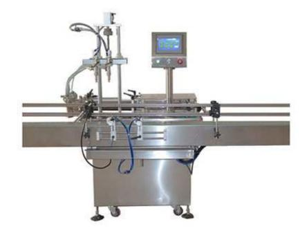
The Automatic Economical Piston Double Nozzles Shampoo Filling Machine is design on the base of the RX-VF, it is also extremely flexible filler capable of filling accurately and rapidly thin and middle viscosity liquids.
