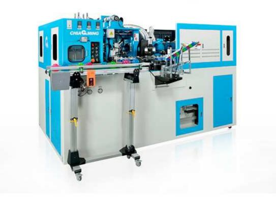
This is a new generation of fully automatic and versatile machine for mass production of PET large volume bottles, oval bottles, flat bottles and jars with volumes up to approximately 6000ml. Ideally suitable for applications where stringent quality requirements have to be met. Suitable for clean lotion, edible oil, detergent, pickle food, etc.
