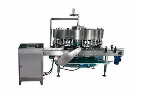
GC12, GC18, GC30 and GC36, these GC series fillers are automatic fixed liquid level type filling machine. The capacity is equals to 14 can/min multiplication by 12 (18/30/36). The filling valve adopts latest filling structure of Italy, fill steady, accurate, high speed and "No dibbing" phenomenon. It is suitable for liquid filling, especially for tin can which already filled solid.
