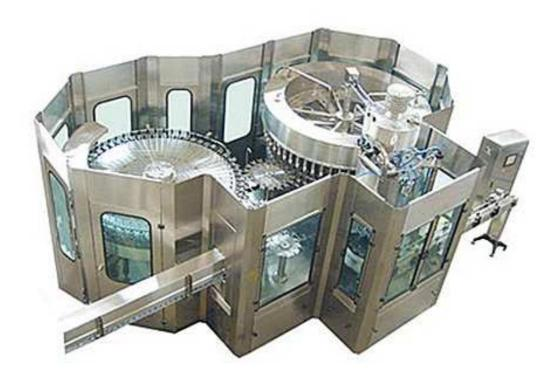
This is high standard advance Touch Screen PLC base Rotary Rinsing Filling Capping Machine. This machine mainly used for washing, filling and capping of Non-Aerated Drink such as Mineral water, Pure Water, Non-Gas Wine Drink, Synthetic Flavoured Juice and so on. The Machine design is shorten the time for the packaging of Pet Bottle, outside contamination and increased the sanitation condition throughout the machine and economical too.
