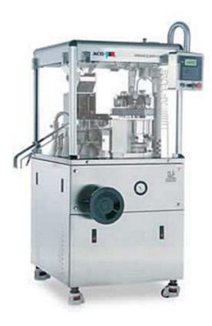
AF-T Lab is a fully-automatic capsule-filling machine that's suitable for laboratories. It ensures greater flexibility to experiment various combinations of dosage forms such that resultant formulations are production-line ready.
