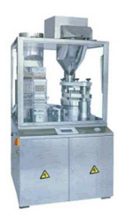
The machine is design for a batch production and retrenchment cost on the basis of NJP-1200A/B/C/D fully automatic hard capsule filling machine. In addition to the function of model NJP-1200A/B/C/D fully automatic hard capsule filling machine, the machine has the rising mechanism that is convenient to clean filling parts. It saves the investment and manpower for enterprise with a batch production.
