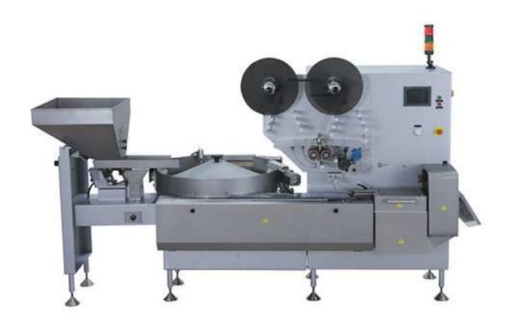
The JH-Z1300 is a horizontal high-speed wrapping machine for hard candy in fin seal (pillow pack). he standard machine is equipped with a sorting station to eliminate sugar dust and chips, a wrapping material feeding system with 2 reel holders and automatic splicer. Two pairs of sealing rollers for the longitudinal seam and a cross sealing unit guarantee a tight pack.
