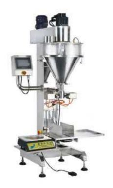
Weighlin automatic auger filler series is special for mini tiny small granules or easy flowing powder, full 304SUS building with high level finish workmanship, various model for different material density, customized design and build for flexible projects in food, chemistry, agriculture, etc industry. Semi-auto work alone or integrated with other upstream or downstream products.
