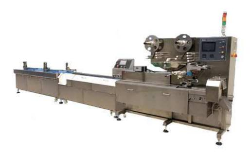
FWC350 Aligner Feeder Flow pack machine is for the automatic feeding and wrapping of small and medium sized products. The machine will automatically arrange products into a single file before automatically feeding them into the wrapping section. The machine will wrap at 300-400 wraps per minute and will speed up and slow down to the speed of the production machines feeding it.
