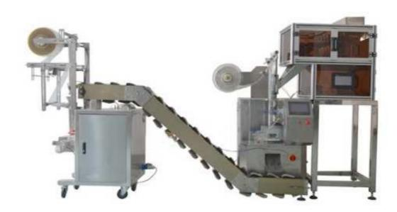
Cost effective: Number of operators: 1 person, total output 2400 bags/hour, 20000 bags 8 hours a day. Traditional hand-made 3~5g low-dose tape labels are inconvenient for packaging outer bags. The inside and outside bags of the triangle bag are equipped with a tape type. The equipment can fully realize your packaging, make your packaging more perfect, and it is more convenient to manage it is good.
