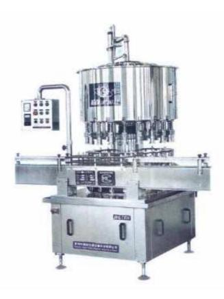
This machine is atmospheric pressure filling machine, rotary continuous filler, cup-type measurement (adjustable), through a specially designed cutting and filling valve drip with microvacuum device (patented technology), Work, no leakage, only Need to replace some of the other accessories, you can meet all kinds of 50-1000ml glass bottles, PET bottles in the automatic filling.
