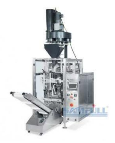
Automatic Volumetric Cup Dosing Packing System apply for regular granular packing machine, such as sugar, soybean, rice, corn, sea salt, edible salt and plastic products, etc.
