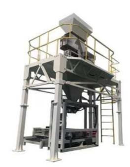
Full automatic open-mouth bag packaging machine is a complete set of machine which is composed of Weighing unit, automatic bag feeding unit and sealing & conveying unit to realize material weighing, automatic bagging, material filling and automatic sealing.
