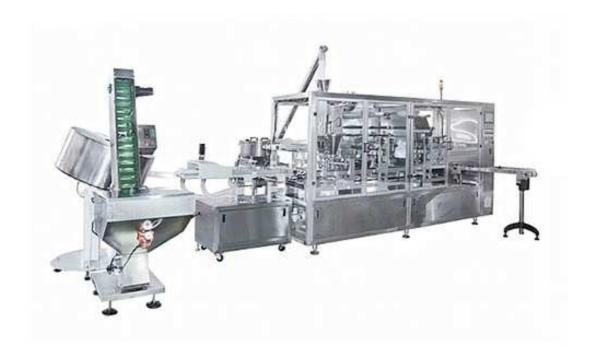
Specially for Dolce Gusto compatible capsules. The Dolce Gusto capsules are automatically sorted and transported to the filling machine for filling, film cutting, and sealing.
