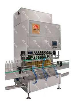
JG inline filling machine especially design for glass bottles, suitable any kinds of edible oil or cooking oil with glass bottles, especially perfect for smaller and medium scale olive oil filling system. It's based on flow meter technology, our flow meter is from china most famous military factory, it's based on roots flow meters technology which make the machine have more high precision and much lower working noise.
