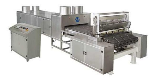
The DRSF series microfilm cooker and servo driven hard candy depositing lines are the advanced equipment for producing hard candies, they are driven by servo motors and controlled by motion controller.
