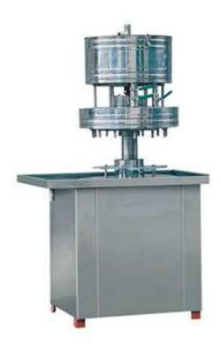
Semi-automatic Water Filling Machine consist of semi-automatic washing machine, semi-automatic Quantitive liquid Bottle Filling Machine, automatic single head screw capping machine, conveyor and motor. This type of machine with the advantage of low investment and easy operation.
