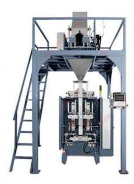
This machine with interrupting movement is indicated to Vertical, Form, Fill and seal (VFFS) high quality three side seal (back seal) and/or Quadro packet machine.
