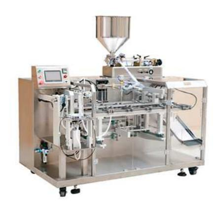
KV-210SGY horizontal premade pouch packaging machine mainly used for premade pouch packing, such as stand up pouch, zipper pouch, spout pouch etc. It is suitable for liquid and paste material. Max speed over 40 bags/min.
