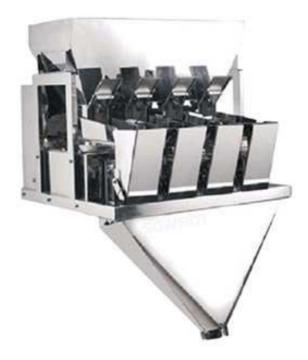
The 4 head high-precision linear combination weigher adopts an all-stainless steel sealed body, which is anti-corrosion and dustproof; the parts in contact with the material (storage bucket, lower hopper, vibrating plate, weighing hopper, etc.) can be quickly disassembled, which is particularly convenient for cleaning. And the food automatic linear scale can be used with various packaging machines and filling machines, and can also be used for semi-automatic packaging.
