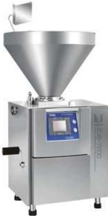
The internal structure principle is to rely on a set of gear pumps driven by a servo motor to accurately push materials to achieve the purpose of quantitative transportation. It can be connected to Sausage Linking System, most automatic sausage clippers to form a sausage line.
