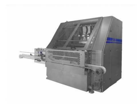
R925 TYPE full automatic cube sugar production and packaging installation by Yılmaz Makina is approved by ISO9001: 2008 quality insurance system. All processes are made without human intervention. The installment is designed for the 24 hour nonstop working principle. And the average capacity is 50000 boxes per day.
