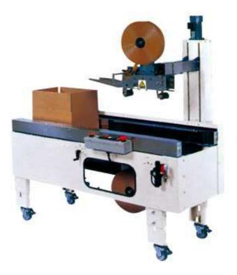
The CU800 is a semi-automatic caser capable of handling A-type cardboard boxes. Product items can be cased quickly by simply being put into opened cardboard boxes. This machine accepts variety of box sizes and the size change can be done in 20 seconds. Valuable options are ready to be equipped like Pre-set Auto Size change, Front-face Printer etc.
