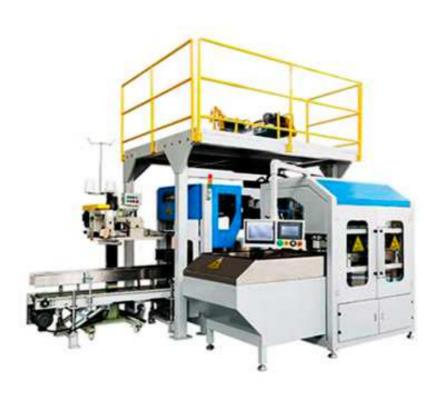
The GW automatic bag placer system is perfect for super store and retail demands by achieving top operational efficiencies, it's design permits the collating of small pouches and vertical arranged separately into the open mouth bag. One row, two row individually or two tows staggered which is by the clients' request.
