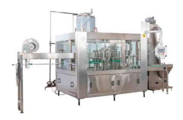
Our newly designed CGF serious monoblook water filling machine is designed for plastic bottle filling, it can suit for PET bottle size between 150ml to 2000ml, can customized to maximum of 3000ml. Genus design of capping design makes different screw cap change into one simple easy torch. On machine surface is only leaving 3 points of bearing support point which makes drainage so easy and without any dirt stain. All bearing have water proof sealing to protect it from getting rust.
