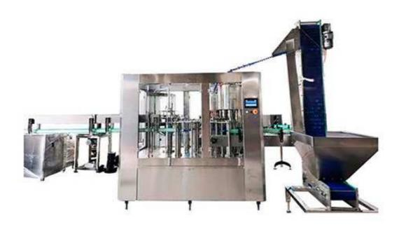
Automatic machine for bottle washing filling and capping, with 18 washing chucks, 18 filling valve and 6 capping heads, production capacity for 500ml mineral water is 4000-6000 bottles per hour. The available bottle sizes for this machine are 300ml – 2000ml.
