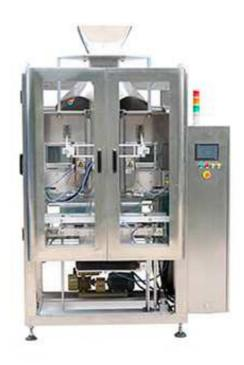
Vertical Packaging Machine GP1020. The max. film width is 1020mm, if to pack 5-10kg powder, this model can solve the problem. The frame of the machine has enough rigidity, which is durable&Long service lifetime. Reasonable structure and each lane separated control also User frinedly& easy for maintenance. It also set up the safety door to protect user safety.
