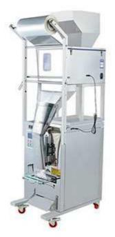
Suitable for packing granules, flakes, bars, powder, such as tea, solid drinks, biscuits, rice, potato chips, shrimp.
