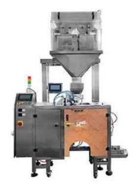
Double Head Weigher Doy Packing Machine is used to fill granular materials into packing containers according to metering requirements and then seal them. It can realize fully automatic weighing, forming, filling and sealing with high efficiency and easy to use. The machine is capable of accurate measurement and strong and beautiful sealing. The excellent quality of Double Head Weigher Doy Packing Machine makes it is playing a bigger and bigger role in the packaging field.
