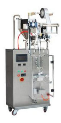
The MK-60YBR vertical form fill seal machine is upgraded on the basis our vertical form fill seal machine MK-60YB, adding a round cutting device while producing the back seam bag. The 4 round corner package appears more beautiful. The MK-60YBR packaging machine is the preferred choice if you have higher quality requirements regarding your packaging.
