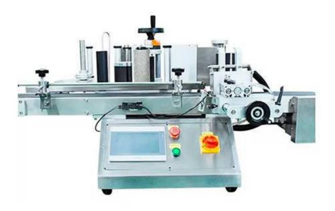
This small tabletop labeling machine is specifically designed, has the characteristic of uniqueness and is used for labeling on circumference and top of the cylinder or on assigned position (labeling on assigned position needs to add accessories). When getting familiar with the table top labeling machine, the machine can be also used for labeling on round container in other industries, such as canned food, round container for tinned food, cosmetics, medicine and so on.
